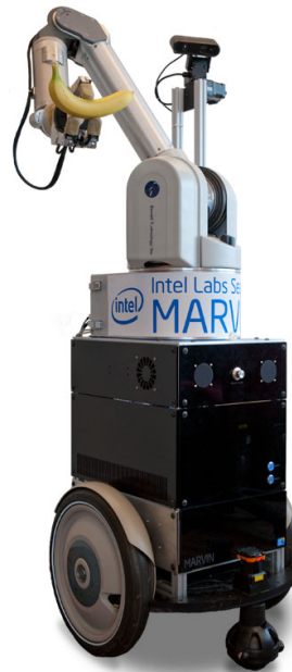
Fig. 1. Photograph of mobile manipulation platform MARVIN, with Electric Field Pretouch-enabled hand. The system includes a Barrett Hand, WAM arm, and Segway base. Each fingertip contains one of our custom electric field sensing boards and 4 sensing electrodes. Another EF sensing board with one transmit electrode is built into the palm, which serves as a hub for aggregating sensor data from the fingertips. The palm also contains a camera, which was not used in the experiments reported in this paper.
