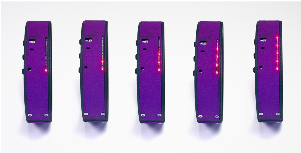
Figure 4.6: The LED display acting as a bargraph, displaying a range of levels.
