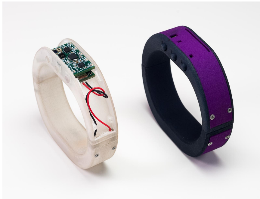
Figure 4.3: Final design of the WristQue prototype, in 3-D printed acrylic (left) and colored laser-sintered nylon (right).
