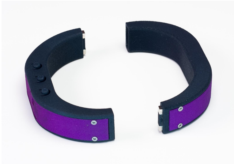
Figure 4.4: The two halves of the WristQue, separated, showing the magnets that hold it together.
