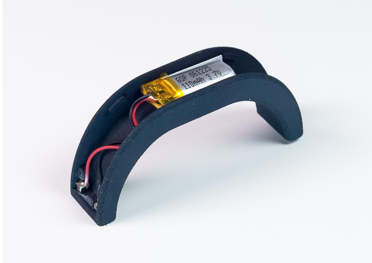
Figure 4.8: The bottom of the WristQue band with the cover removed, showing the battery inside.
