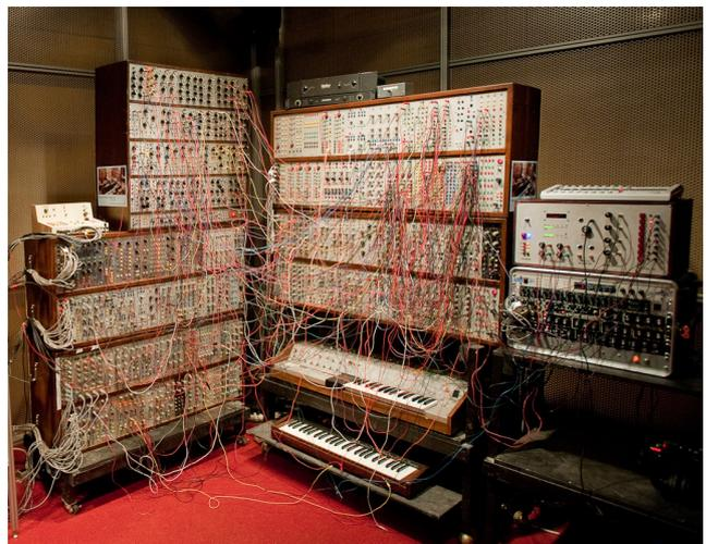
Figure 1: Paradiso's modular analog synthesizer.
