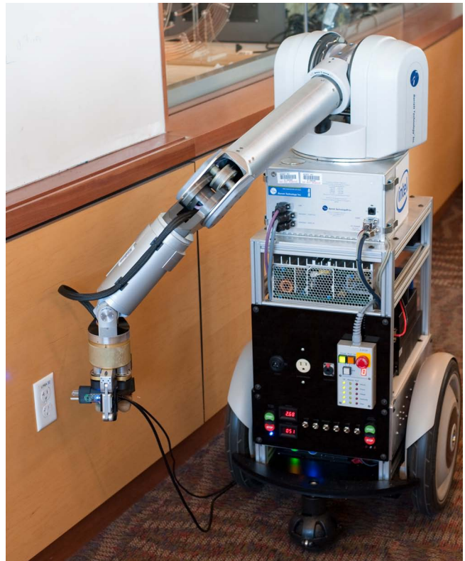
Fig. 1. The MARVIN Mobile Manipulation Platform is able to plug itself in to a standard U.S. electrical outlet. The outlet and building wiring are completely standard and unmodified; the robot’s plug has been instrumented to sense the 60Hz AC electrical emissions from the outlet. After the robot has navigated to the vicinity of the outlet, the plugging in process is guided entirely by measurements of these electrical emissions; the outlet is not sensed visually at all.
