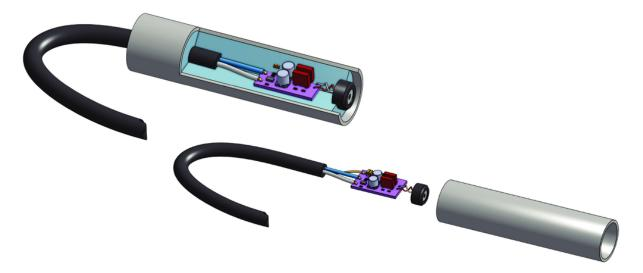
**Figure 4.6:** Weather-proof omnidirectional microphone (v2), cut-away and exploded views
