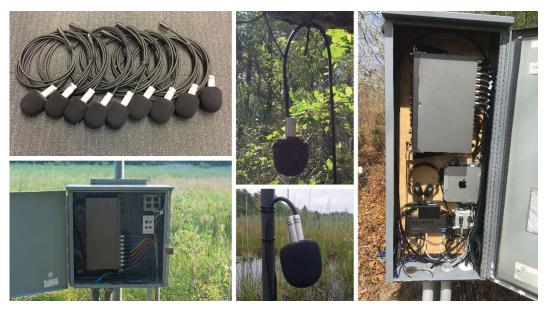
**Figure 4.4:** Audio installation at the Impoundment: microphones ready for deployment and in the field, main base station (right), satellite box (lower left).
