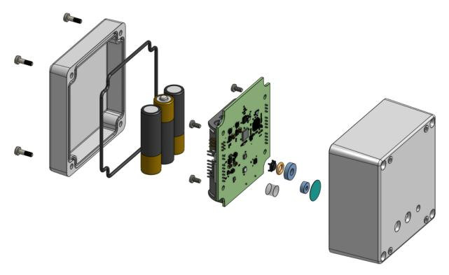
Figure 3.3: First-generation sensor node assembly, exploded view
