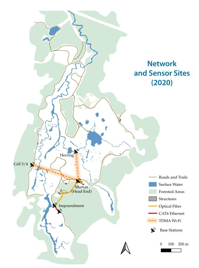
Figure A.6: Network infrastructure and sensor site names (2020).
