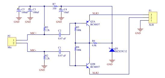
Figure 4.7: Weather-proof omnidirectional microphone (v2) schematic
