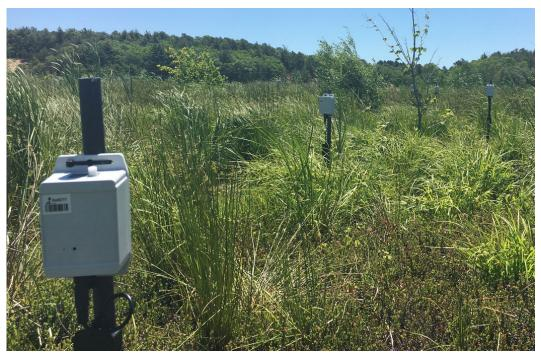
Figure 3.11: Second-generation nodes in the microtopography cluster.
