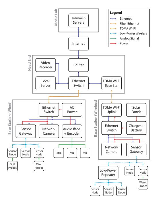
**Figure 3.1:** Schematic diagram showing the physical structure of the Tidmarsh sensor network as of the summer of 2020. Note that there are more base stations, sensor nodes, cameras, etc. than represented here.
