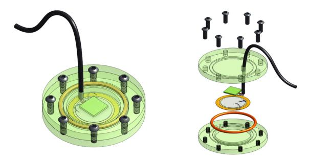
Figure 4.8: Hydrophone prototype (v1), assembled and exploded views
