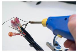
(o) Step 15. Solder the Ground Wires
