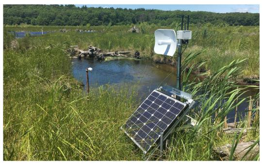
Figure 3.7: The off-grid base station at the herring site.
