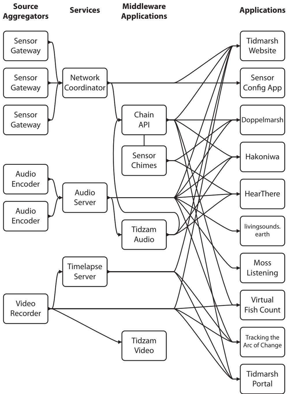
**Figure 3.2:** Data flow from sensor network inputs, through infrastructure services, to a selection of applications.
