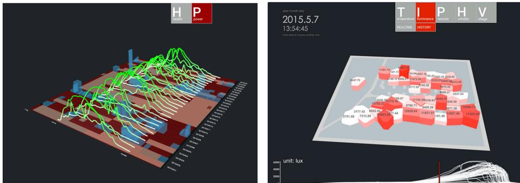
**Figure 6.6:** MarshVis displaying base station power (left) and illuminance across the sensor network (right).
