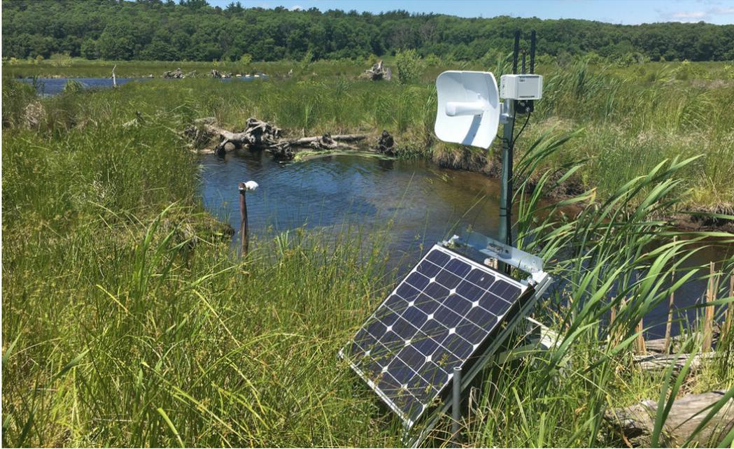
**Figure 3.7:** The off-grid base station at the herring site.
