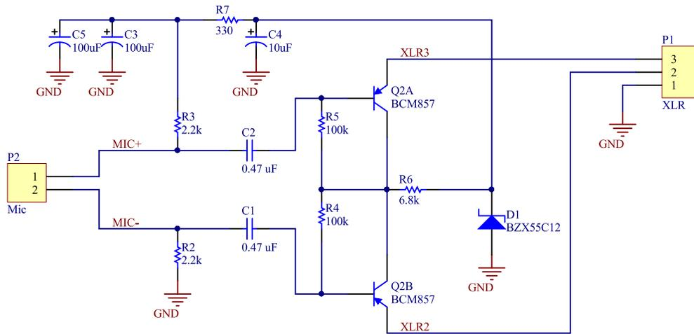
**Figure 4.7:** Weather-proof omnidirectional microphone (v2) schematic
