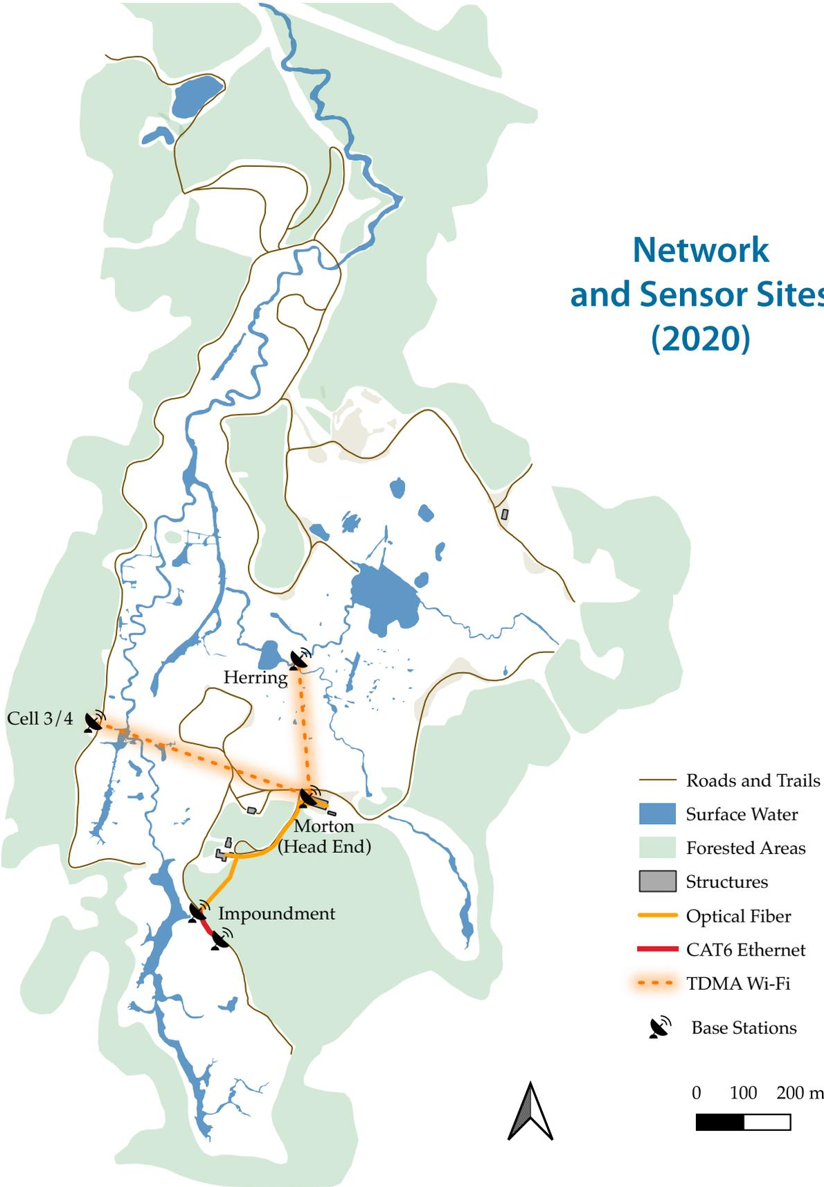
Figure A.6: Network infrastructure and sensor site names (2020).
