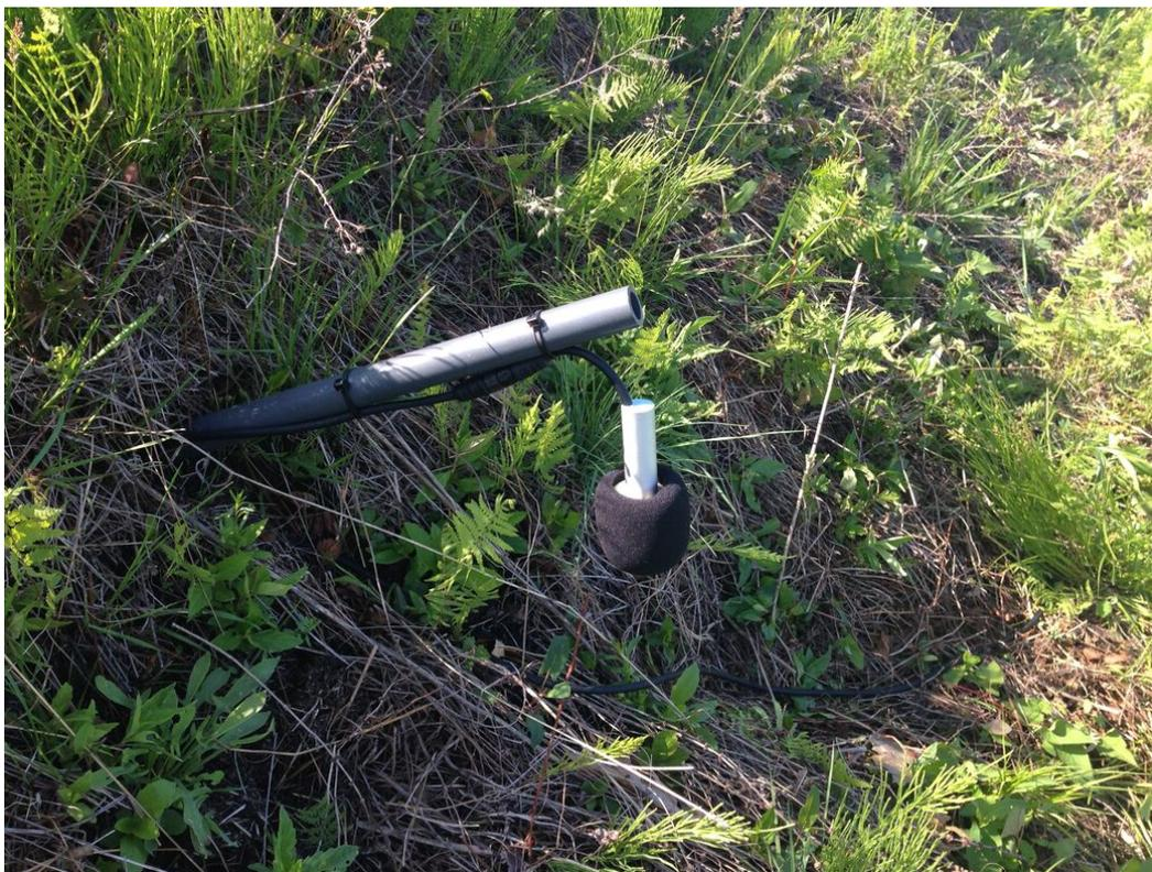
**Figure 4.3:** A microphone in cell 3.
