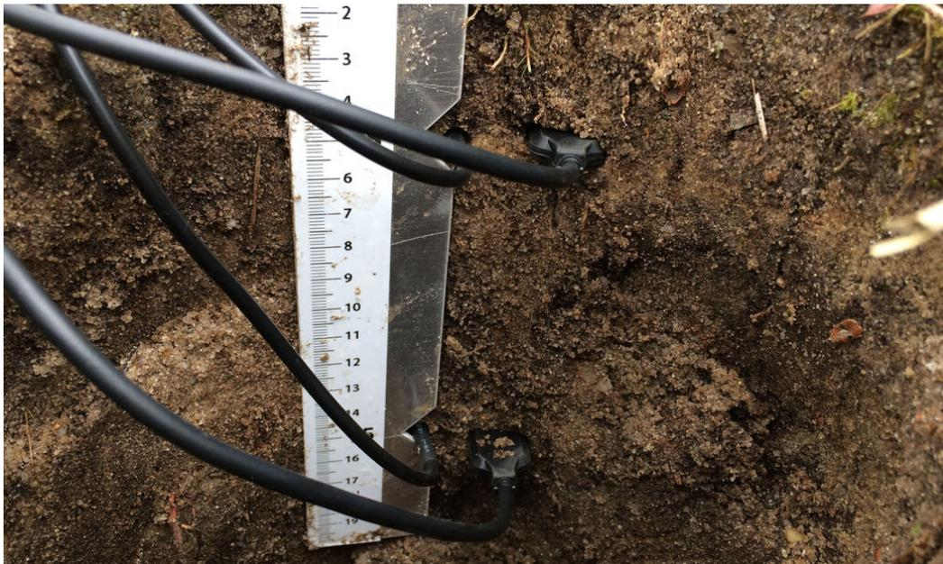
**Figure 5.1:** Soil moisture probes inserted into the side of a hole, with installation jig
