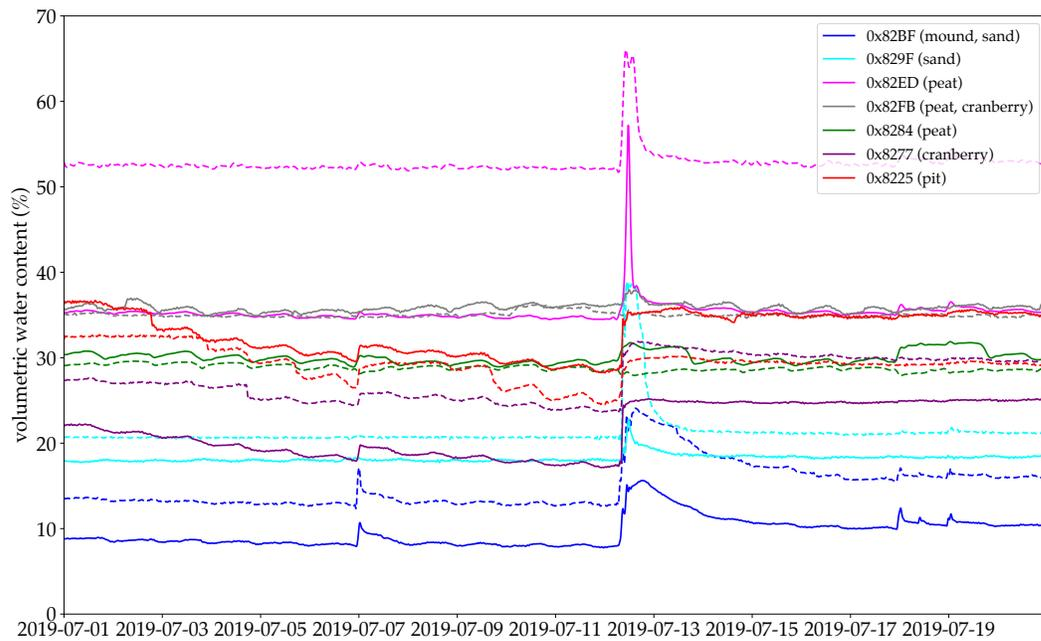
**Figure 5.3:** Soil moisture preceding and following a significant July storm. Solid lines are probes at 5 cm depth; dashed lines are at 15 cm depth.
