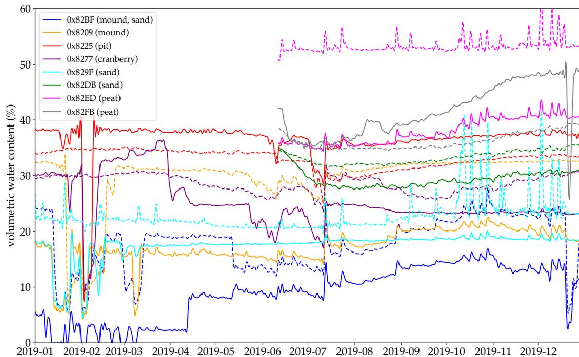
**Figure 5.2:** Soil moisture from selected sensors across Tidmarsh, 2019. Solid lines are probes at 5 cm depth; dashed lines are at 15 cm depth.
