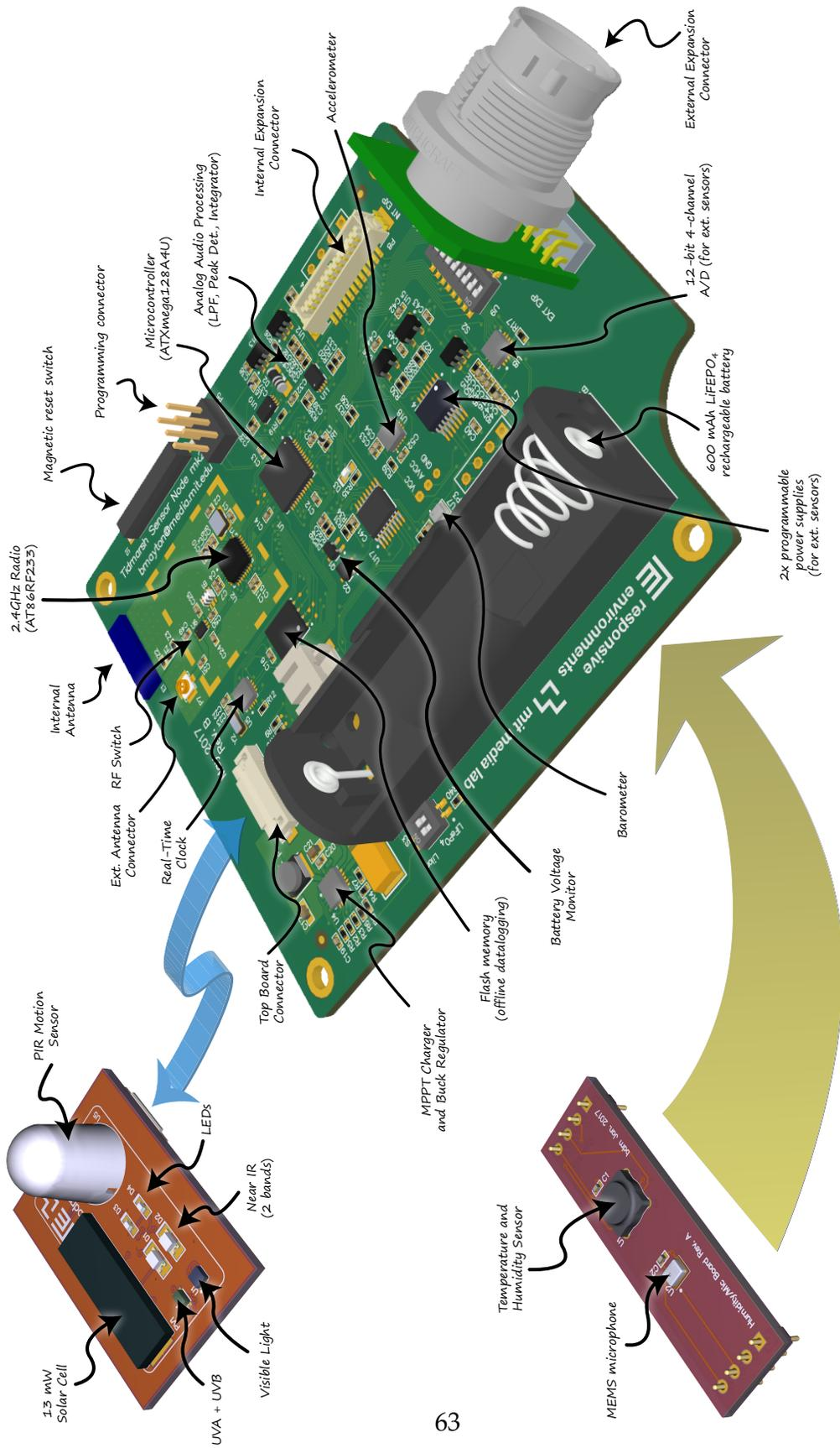
Figure 3.5: Second-generation sensor node electronics.
