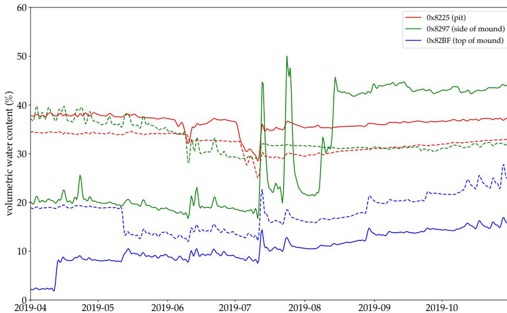
**Figure 5.5:** Soil moisture from different microtopographical aspects. Solid lines are probes at 5 cm depth; dashed lines are at 15 cm depth.
