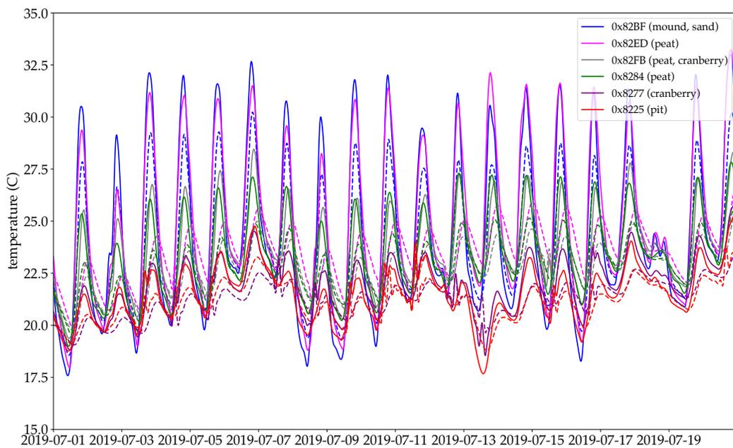
**Figure 5.4:** Soil temperature preceding and following a significant July storm. Solid lines are probes at 5 cm depth; dashed lines are at 15 cm depth.
